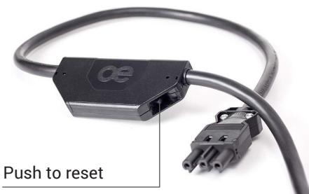
A thermal bimetallic strip, which has the advantage of being immune to high inrush currents and line transients, is heated by overcurrent and deflects thereby releasing the latch mechanism. The contacts open even if the reset button is manually held in the closed position. This is known as a trip-free mechanism. The contacts open and close with a positive snap action and the tripped state is clearly indicated by the extended projection of the reset button.
